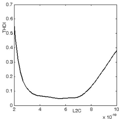
Fig. 10 Total harmonic distortion factor of the supply current versus product  $L2C$  for  $C = 0,1\mu F$
