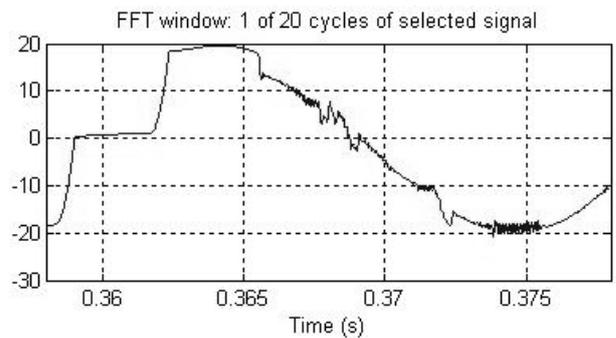
Fig. 11 Dynamic response of the active power filter
