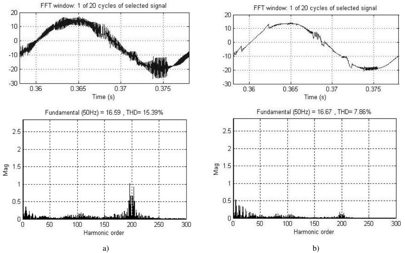
Fig. 8 Power supply current waveform and its harmonic spectrum: a) unfiltered ; b) filtered
