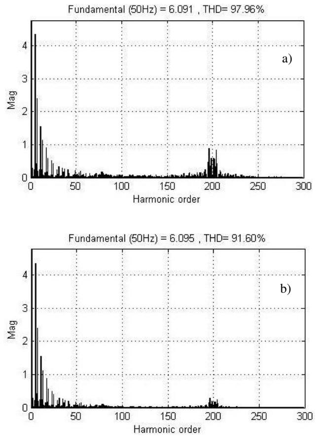
Fig. 7 Harmonics spectra of the current provided by the active power filter: a) before interface filter; b) after interface filter
