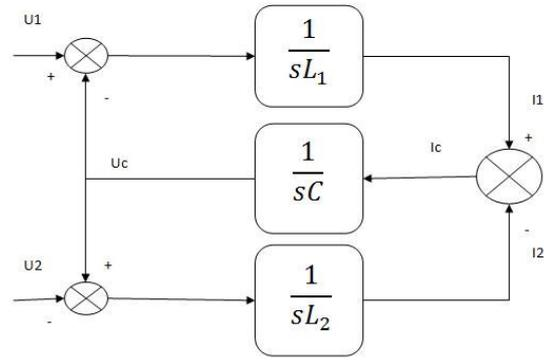
Fig. 4 Block diagram of the second order interface filter
