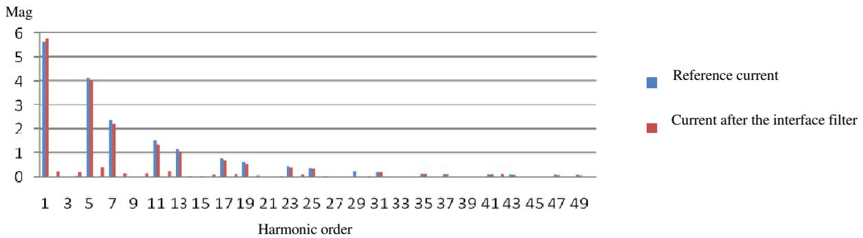
Fig. 9 Comparison between the harmonic spectra of the reference current (to be compensated) and the current after the interface filter
