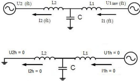
Fig. 3 Equivalent configurations of the interface filter at the fundamental and harmonic frequencies
