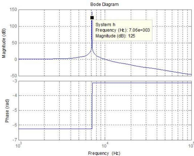
Fig. 5 Frequency response of interface filter
