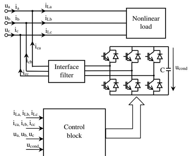
Fig. 1 Basic structure of a three phase active power filter
