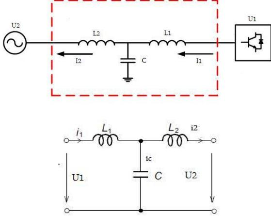
Fig. 1 Equivalent schema of the LCL interface filter
